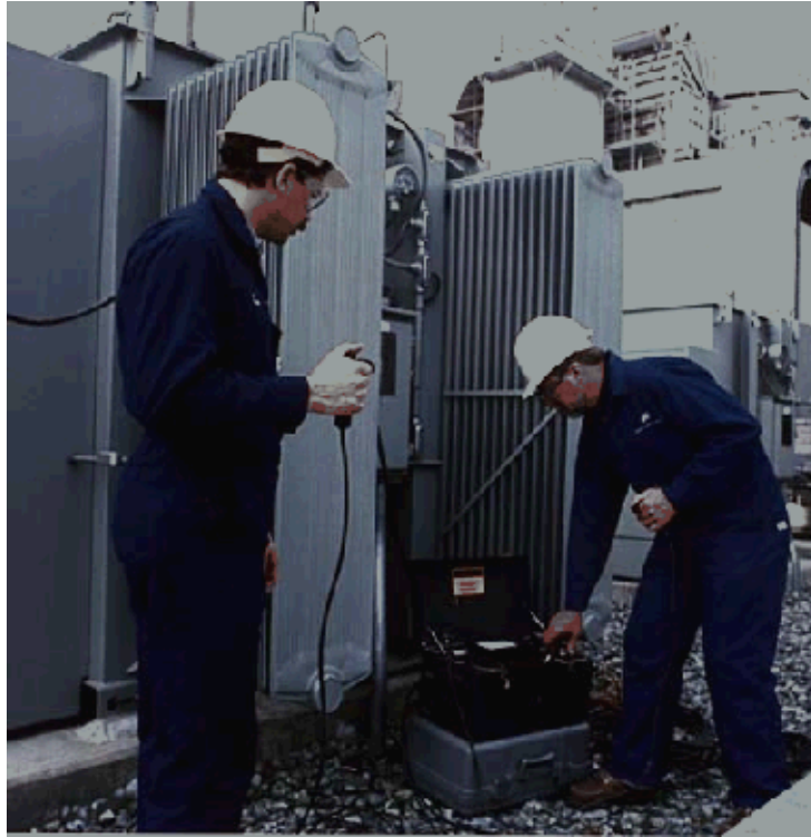
Figure 6-2—Insulation power-factor testing
