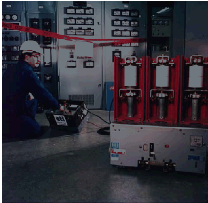
Figure 6-1 — Circuit breaker high-potential testing
